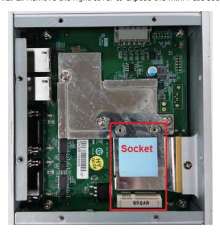
**STEP 3:** Insert the wireless module card into the socket at an angle.
