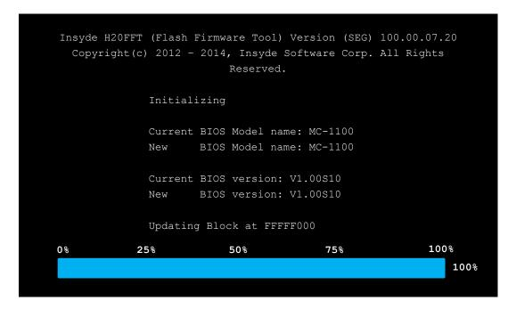
6. When the upgrade is finished, the computer automatically reboots. You may check the BIOS version on the Main page of the BIOS setup utility.
