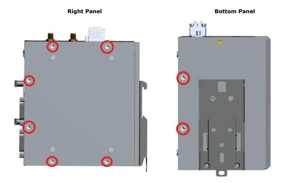
**STEP2:** Remove the right cover to expose the mini-PCIe socket.
