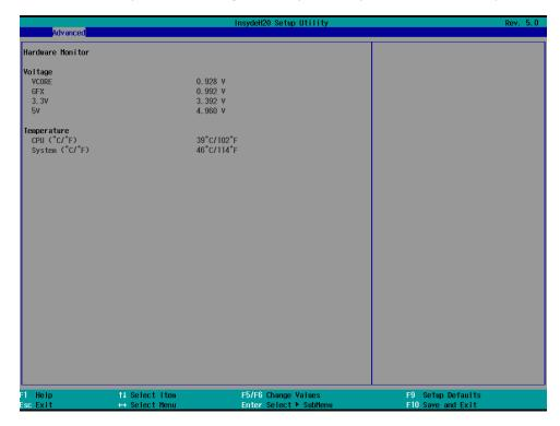
Note that the voltage values vary depending on the model. The temperature readings shown on the screen are within  $\pm 5\%$  of the actual readings. However, the temperature readings are only valid when the ambient temperature is above 0°C.
